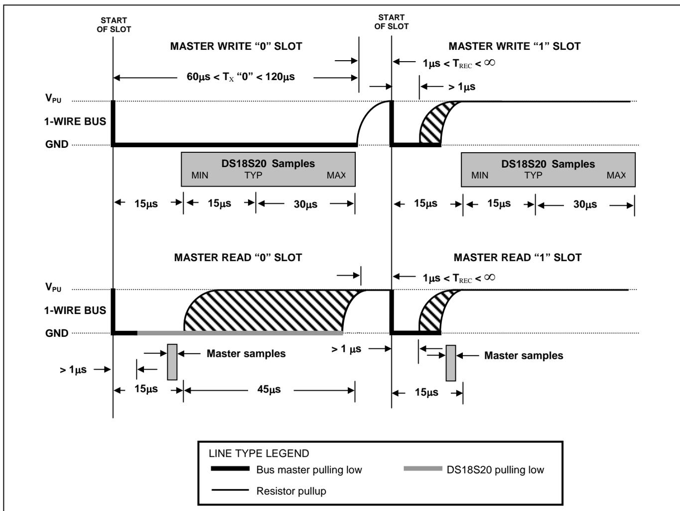
Figure 12. Detailed Master Read 1 Timing
